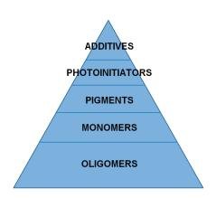
Figure 3: Typical formulation of a UV curable ink
