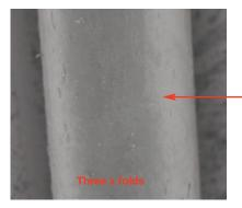
Ink film still fully adhered to substrate No sign of cracking after three folds
