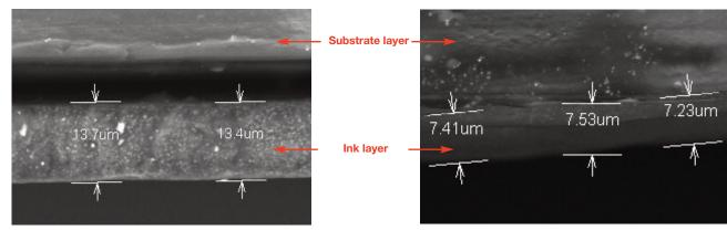
Figure 7: White ink film printed with double printbar
