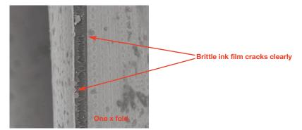
Figure 9: 8 µm ink film printed with single printbar of Xaar 1002 GS6 (200x magnification)
