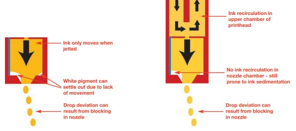
Figure 4: Ink sedimentation in end-shooter printhead
